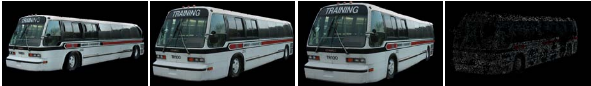
Figure 6: A reconstruction from a single reference view. This model has over 400k points, upsampled in under a second. While the bus has simple geometry, it is challenging because it is highly specular, and many surfaces have little texture. Again we show the initial point cloud on the right.
