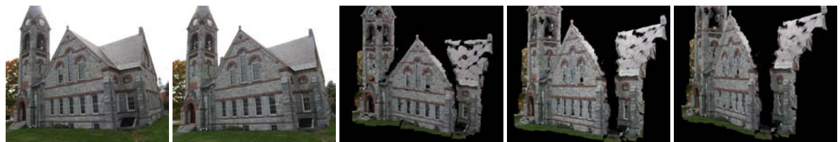
Figure 9: A dense reconstruction obtained from only 2 views through our entire pipeline. Because there are only two views, we computed the initial point cloud with Bundler in about 30 seconds. Although Bundler provided depths for only about 0.1% of the pixels in each image, our algorithm produced an accurate model composed of more than a million points in under a second.
