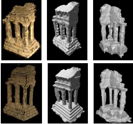
Figure 3: Top: A point cloud computed with our algorithm, and two views of a smooth surface created using Poisson surface reconstruction with depth=8 . Bottom: the same test performed on a dense point cloud from PMVS ( level=1 , csize=1 ).
