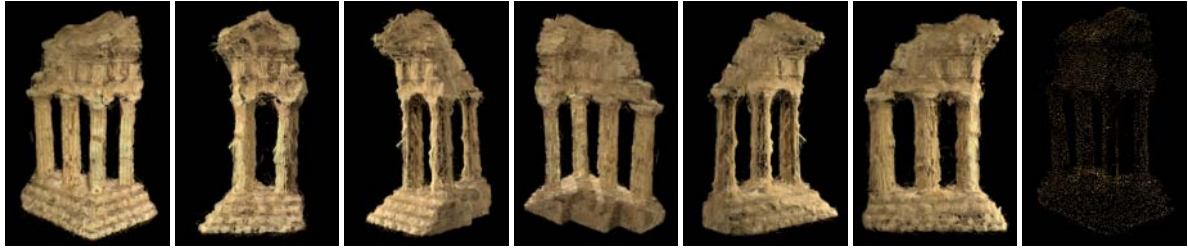
Figure 5: A full reconstruction of the temple model [SCD*06a]. We merged the depth maps from 6 reference views to produce nearly 400k points. Upsampling took less than a second. On the right, we show the initial sparse point cloud.
