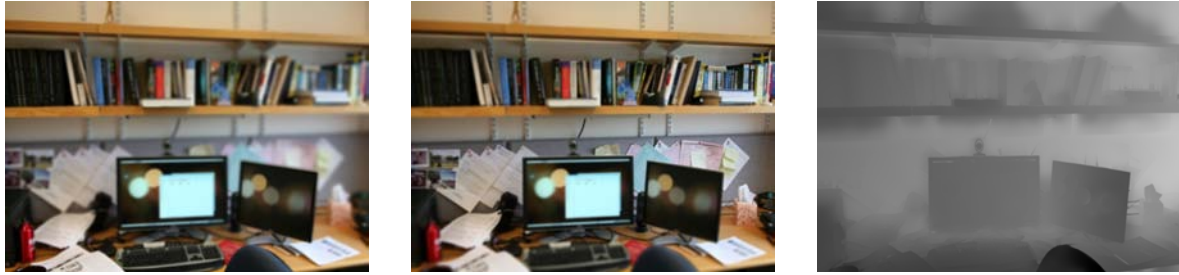
Figure 11: Left: An image of an office, refocused on the chair. Middle: The same image, refocused on the wall behind the right monitor. Right: The depth map.
